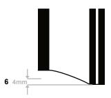
**6** - Steps between the top and bottom pane of glass of more than 4mm.
