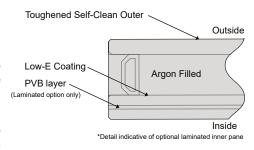
This product has a Low-E coating typically on the internal pane. Low-E glass types can produce transient visual effects such as haze or transparent film effect in certain lights - this is not a fault with the product.
