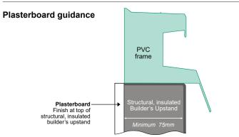
Finish plasterboard at the top of the structural, insulated builder's upstand. Do not cover any of the PVC frame. For more information see TB409.
